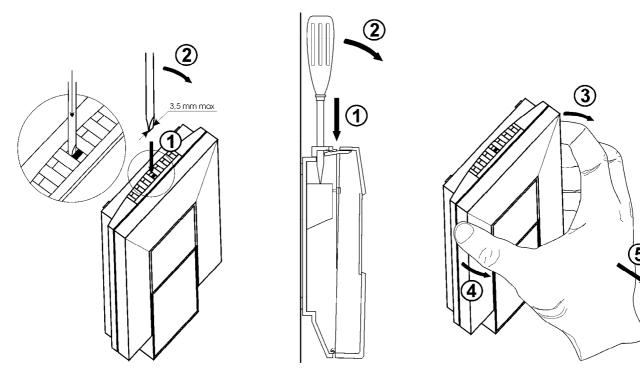
Figure2: Device demounting
