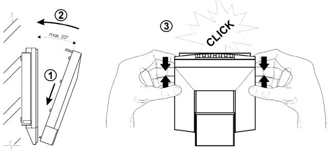
Figure1: Device mounting
